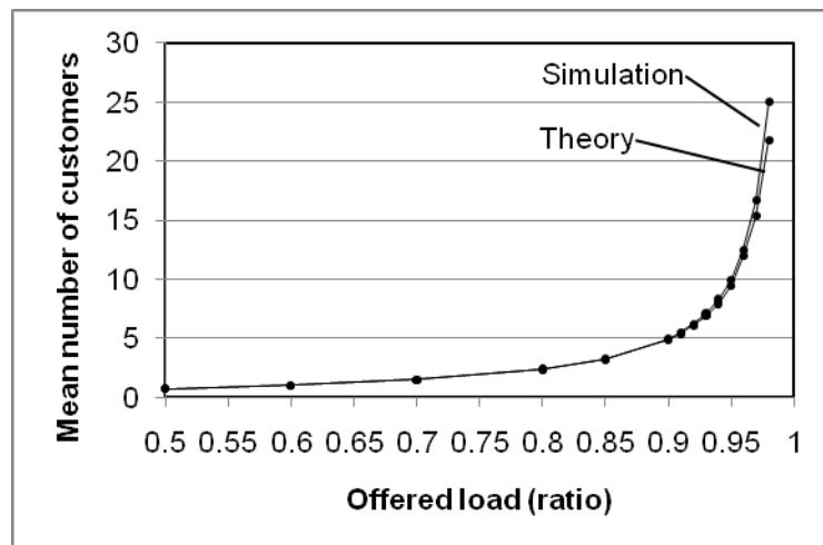
The absolute magnitude of relative error is less than for the M/M/1 simulation. This is because there is less variability in the M/D/1 case (deterministic service, which has variance = 0) than the M/M/1 case (exponential service time with non-zero variance).
