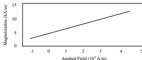
Fig. 1. Magnetization as a function of applied field.
