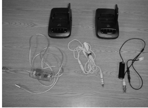
Figure 8 – Photograph of equipment used in demonstration; clockwise from top-left: Clover 2.4 GHz wireless Audio/Video Sender, 1/3 inch submersible color bullet camera, microphone, D-Link DSB-V100 USB video capture device
