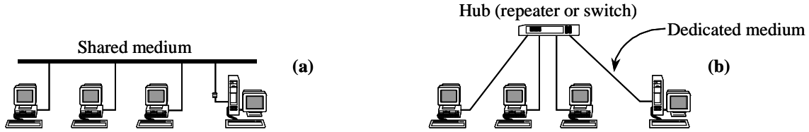
Figure 2 - Examples of shared-medium and dedicated-medium networks
