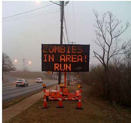
16 17 Figure 2 A compromised DMS from an online guide on exploiting DMSs [67]
