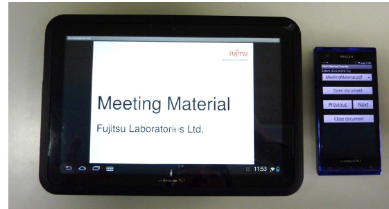
Figure 8. When there are a tablet computer and a smartphone in the meeting room, the document viewer service is installed into the tablet computer and the slide controller service is installed into the smartphone.
