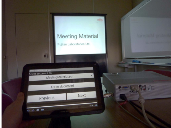
Figure 9. When there are a tablet computer and a projector in the meeting room, the document viewer service is installed into the projector and the slide controller service is installed into the tablet computer.
