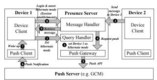
Figure 2. Integration with push notification for mobile devices
