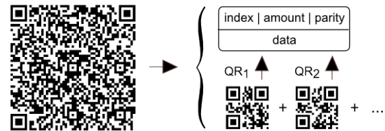
Figure 2. A long message is split over multiple barcodes and a custom header is added to each barcode to overcome the limitations of a QR code’s structured append mode.
