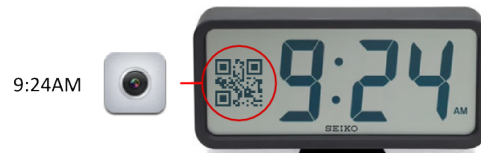
Figure 1. This clock presents the time in two formats – a dynamic barcode also allows a computing device to accurately read the current time.
