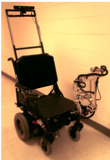
Fig. 7. The Wheelchair-Mounted Robotic Arm system (WMRA) that would be used to assist physically-challenged individuals.
