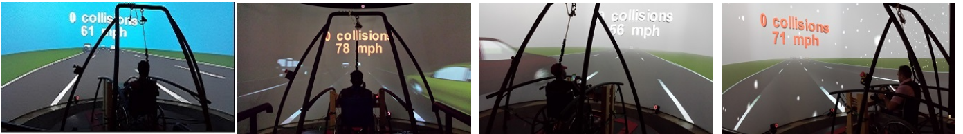
Fig. 1: Four Participants in the Driving Simulator in Different Environmental Conditions (Day time, Night time, Fog and Rain/Snow)
