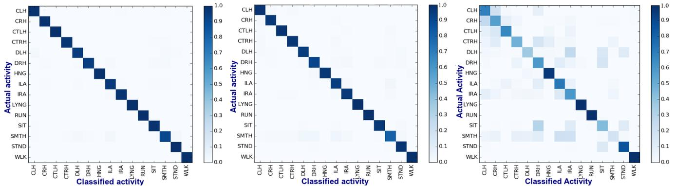
Figure 7. Confusion matrix for evaluation by Same user 10-fold cross-validation method (left), Cross user 10-fold cross-validation method (middle), Cross user Leave-one-out cross-validation method (right)
