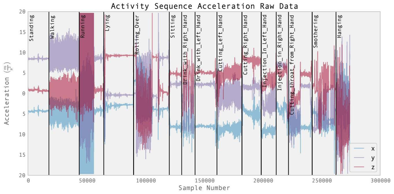
Figure 3. Recorded accelerometer readings throughout an activity sequence from the Shimmer device secured to participants left hand. The blue series denotes the  $x$  component, red shows  $y$ , and purple shows  $z$ .
