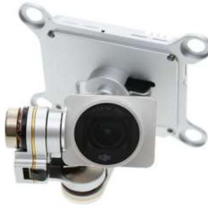
**Figure 4.** DJI 4K camera with a 8.8 mm/24 mm; f/2.8; 1" CMOS; 20 MP) for RGB capture point Anopheline habitat imaging in the Akonyibedo village epi-entomological, intervention, study site.
