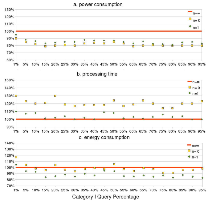
Fig. 8. Relative quantity of power, processing time and energy consumption under workloads with different category I to II query ratios.
