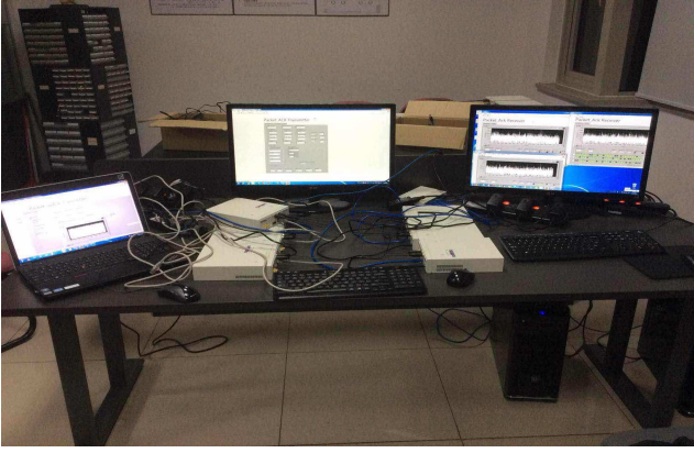
Fig. 2: Experiment prototype system with 7 USRPs
